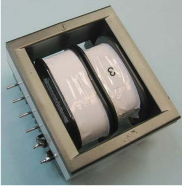
Figure 27. Photo of Integrated LLC Transformer with Separated Primary and Secondary Windings.
