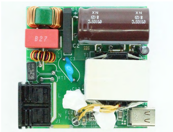
Figure 5 DER-601 – 60 W wide-range USB PD charger (5 V – 20 V output) showing high efficiency across load. InnoSwitch3-CP INN3279C-H215. 60 W adapter design—no heatsink required.
