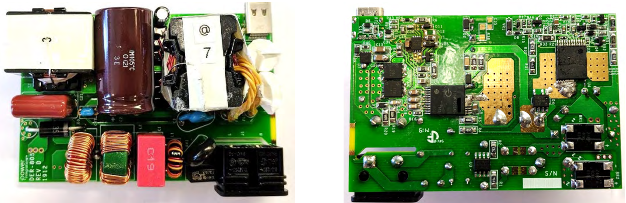
Figure 6 DER-805 – 100 W wide-range USB PD + PPS charger (5 V – 20 V output) with no- heatsink required. InnoSwitch3-Pro INN3370C-H302.
