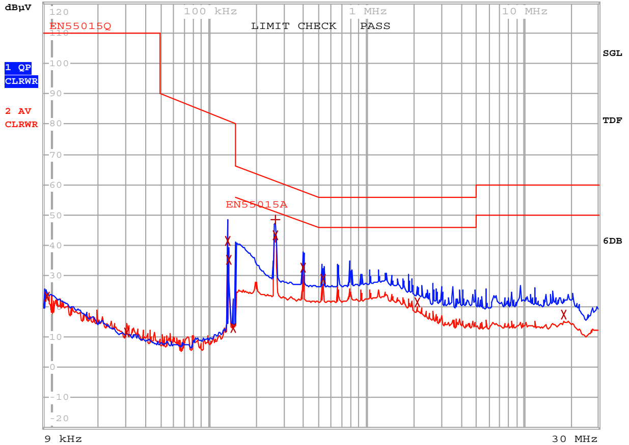
Figure 66 – Conducted EMI, ~48 V LED Load, 115 VAC, 60 Hz, and EN55015 B Limits.
