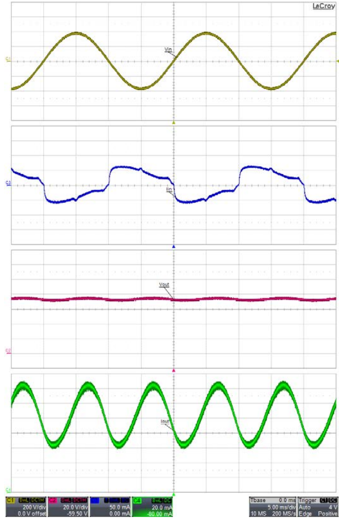
Figure 40 – 265 VAC / 50 Hz, Nominal V_{LED} Load. Ch1 (Yellow): V_{IN} , 200 V / div. Ch2 (Red): V_{OUT} , 20 V. Ch3 (Blue): I_{IN} , 50 mA / div. Ch4 (Green): I_{OUT} , 20 mA / div. Time Scale: 5 ms / div.
