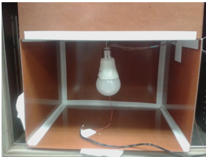
Figure 18 – Thermal Unit Thermocouple Measurement Set-up.
