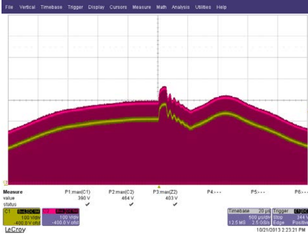
Figure 217 – Differential Line Surge at 500 V / 90°. Peak Drain Voltage Recorded is 464 V. Ch1: V_{BULK} ; 100 V / div. F1: V_{DRAIN} ; 200 V / div. Time Scale: 500 \mu s / div.
