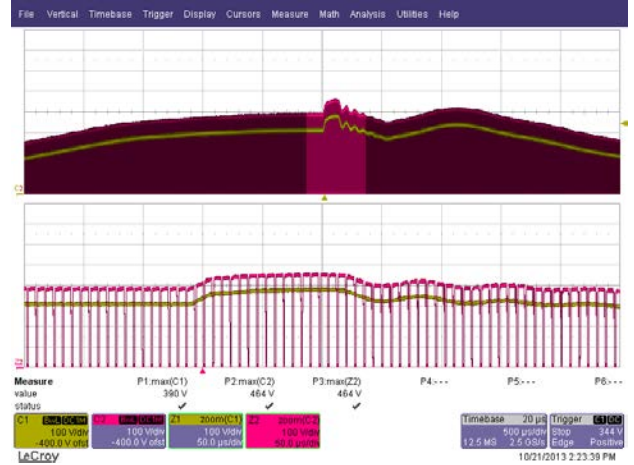
Figure 218 – Differential Line Surge at 500 V / 90°. Peak Drain Voltage Recorded is 464 V. Ch1: V_{BULK} ; 100 V / div. F1: V_{DRAIN} ; 200 V / div. Time Scale: 500 \mu s / div. Zoom time Scale: 50 \mu s / div.
