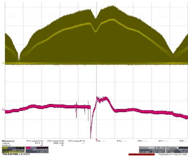
Figure 92 – 265 VAC / 50 Hz, 36 V Load, V_{DS} = 611 V_{PK} (+) 500 V Diff. Line Surge at 270°. Ch1: V_{BULK} , 100 V / div. Ch2: V_{DS} , 200 V / div. Time Scale:200 \mu s / div. Zoom Time Scale:20 \mu s / div.
