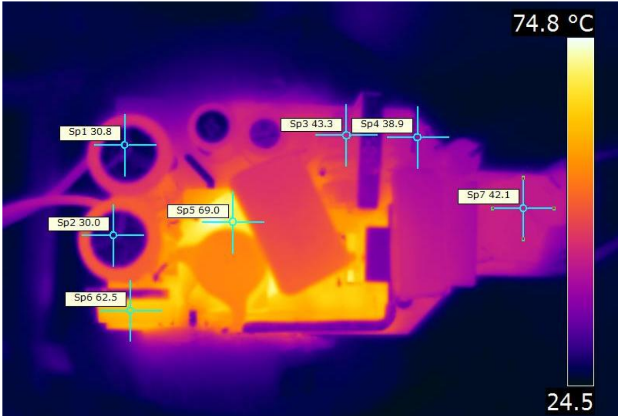
Figure 22 – Open Frame Thermal Scan
