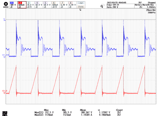
Figure 54 – INN3947CQ Drain Voltage and Current. 60 V DC , 1.333 A Load. CH1: V DS , 100 V / div. CH2: I D , 500 mA / div. Time: 10 μs / div.
