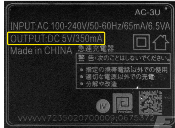
Charger nameplate rating
