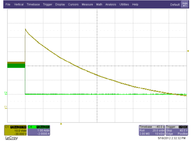
Figure 34 – 300 VAC / 63 Hz, Load is Removed; Ch1: V_{OUT} , 10 V / div. Ch4: I_{OUT} , 1 A / div., 20 s / div.
