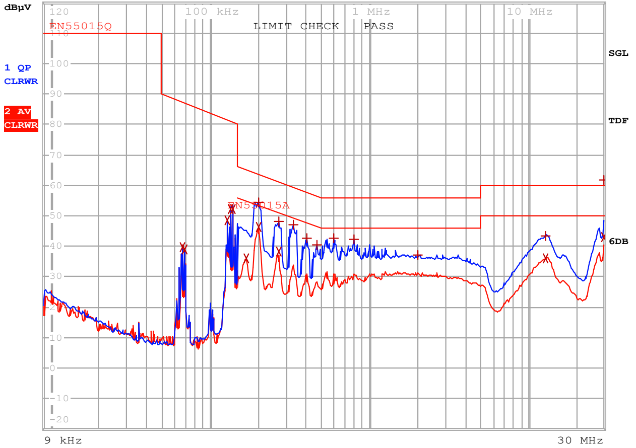
Figure 43 – Conducted EMI, Maximum Steady State Load, 230 VAC, 60 Hz, and EN55015 Limits. 3-Wire Configuration (L-N-Earth), Chassis Floating.
