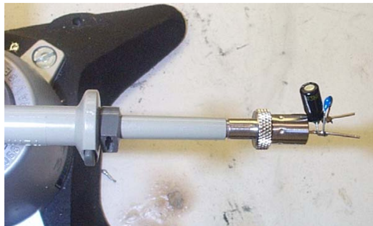
Figure 29 – Oscilloscope Probe with Probe Master 4987BA BNC Adapter (Modified with Wires for Probe Ground for Ripple measurement and Two Parallel Decoupling Capacitors Added).
