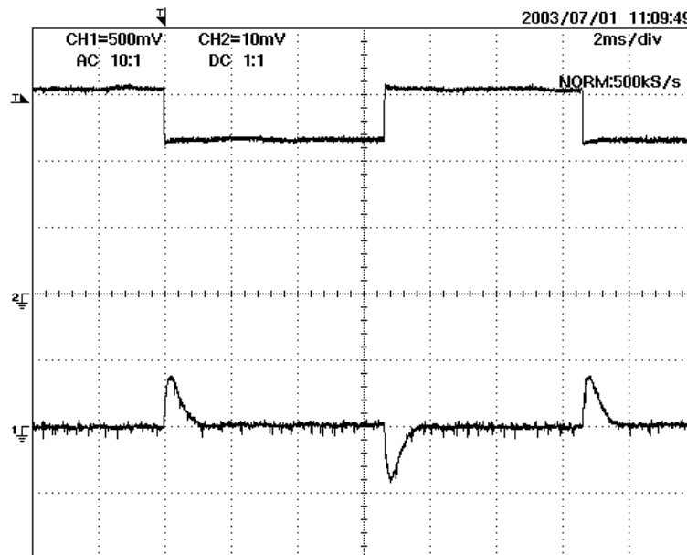
Figure 20 – 58V input. 8V2 rail load transient response (Upper – 8V2 rail current at 0.5A/div, Lower – AC coupled 8V2 rail voltage at 500mV/div)
