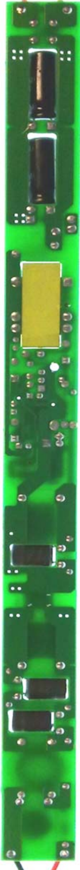
Figure 2 – Populated Circuit Board Photograph (Bottom View), Board Dimensions 260.44 mm x 19.53 mm
