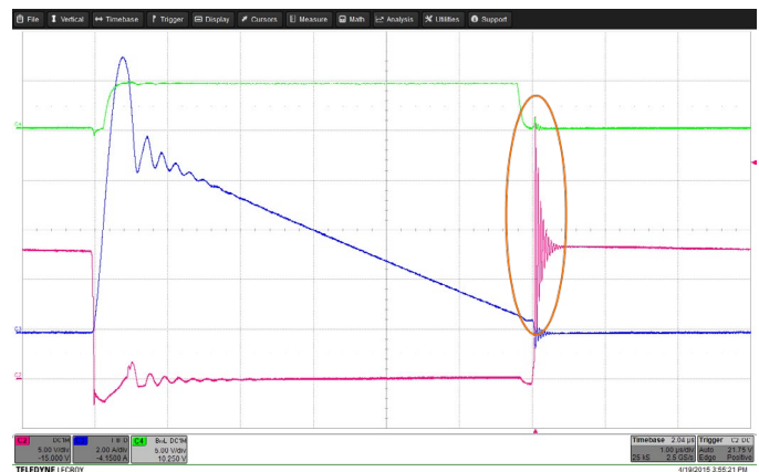
Figure 25. Measure the Frequency of Oscillation of the SR FET VDS During Turn-Off Ringing (encircled) to Solve for SR FET Snubber Values.
